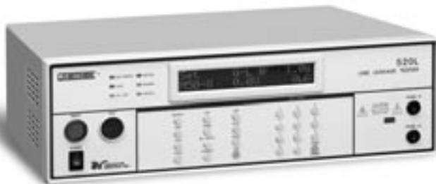
**(Figure 4) LINECHEK™ Model 520L Automated Line Leakage Tester.**
